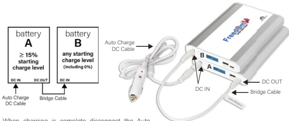
When charging is complete disconnect the Auto Charge DC Cable from the vehicle and the battery.
